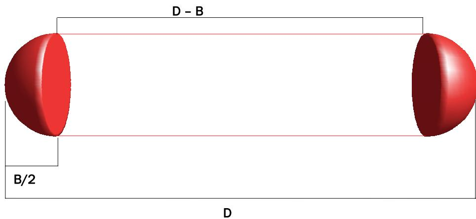
Length of cylinder = displacement sphere =  $D - B$
