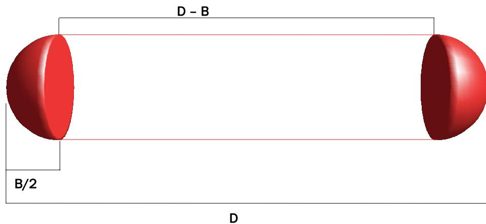
Length of cylinder = displacement sphere =  $D - B$
